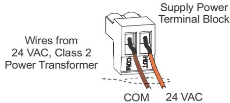
**IMPORTANT:** The 24 VAC power should not be shared with other network devices. Sharing power with other network devices may cause noise, interference, and ground loop problems. You may damage the controller by sharing power with other devices.
