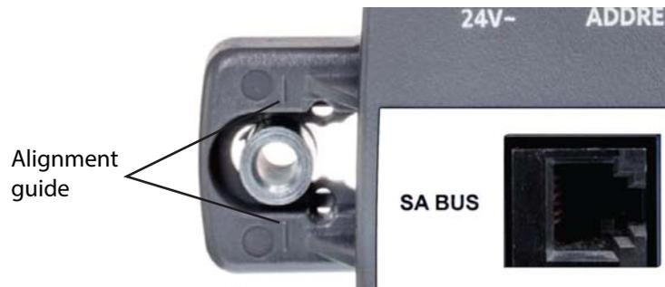
5. Secure the self-drilling No. 10 screw through the captive spacer with a power screwdriver and 100 mm (4 in.) extension socket. Otherwise, use a punch to mark the position of the shoulder washer, and then drill a hole into the VAV box using a 5/16 in. drill bit. Insert the mounting screw and tighten it against the spacer.
