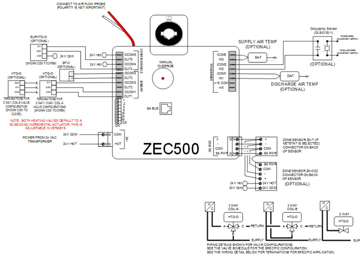
**Sequence of Operation for Incremental Control Wiring Example**
