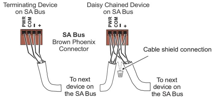
Stranded, 4-Wire consisting of 2 twisted pairs of shielded cables.
