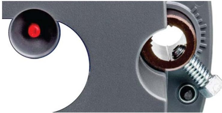
9. If the damper for a 45° or 60° box closes CCW, rotate the coupler to the CW mechanical limit. If the damper for a 45° or 60° box closes CW, rotate the coupler to the CCW mechanical limit. This action sets the open end-stop; the closed end-stop is set by the closed damper.
